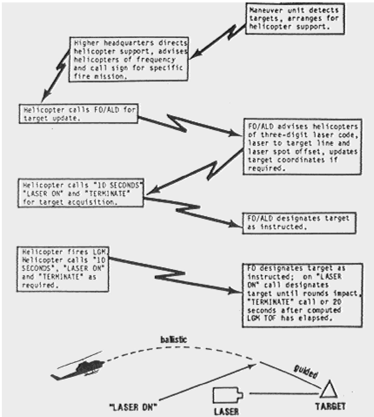
Figure B-8. Procedures for Helicopters with LST/LGM
