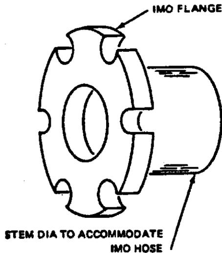
TO ENABLE PIPES OF RECEPTION FACILITIES TO BE CONNECTED WITH THE SHIP'S DISCHARGE PIPE LINES FOR THE RESIDUES FROM MACHINERY BILGES, LINES SHALL BE FITTED WITH A STANDARD DISCHARGE CONNECTION IN ACCORDANCE WITH THE FOLLOWING TABLE:
