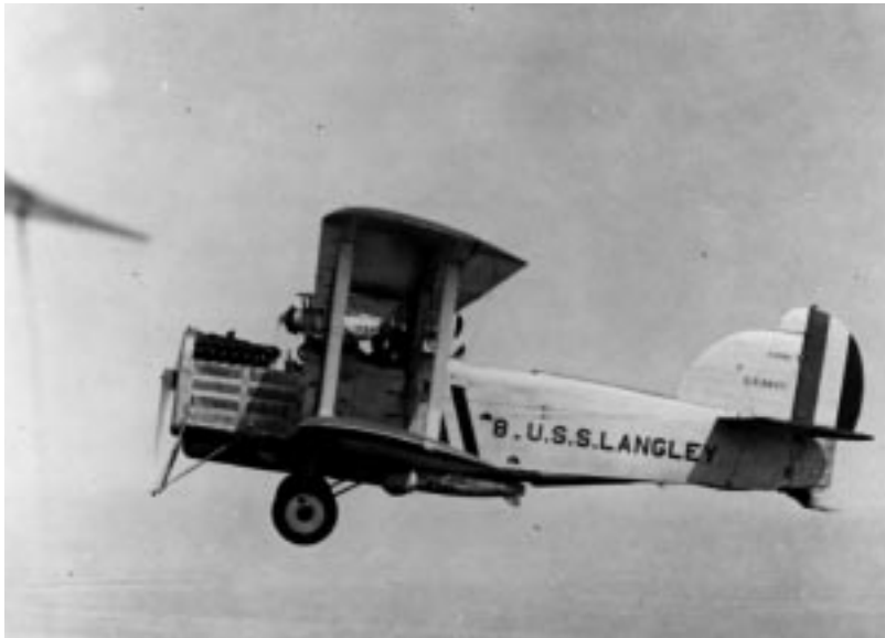
DT-2 from USS Langley with torpedo and rigged parachute, 1926.
