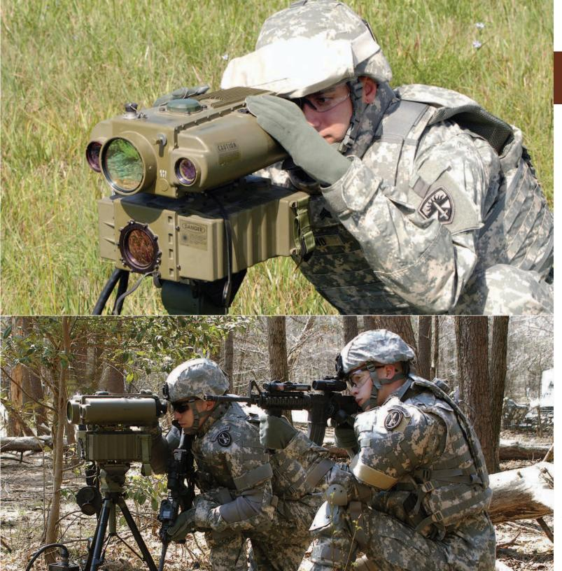
Lightweight Laser Designator Rangefinder (LLDR) AN/PED-1 & AN/PED-1A
