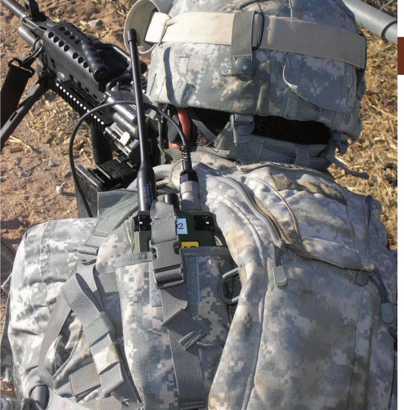
**Joint Tactical Radio System** Handheld, Manpack, Small Form Fit (JTRS HMS)
