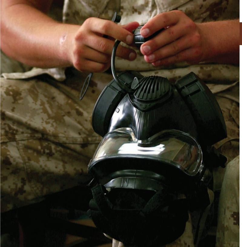
Joint Service General Purpose Mask (JSGPM) M-50/M-51
