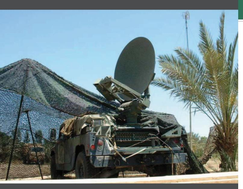
Secure Mobile Anti-Jam Reliable Tactical Terminal (SMART-T)
