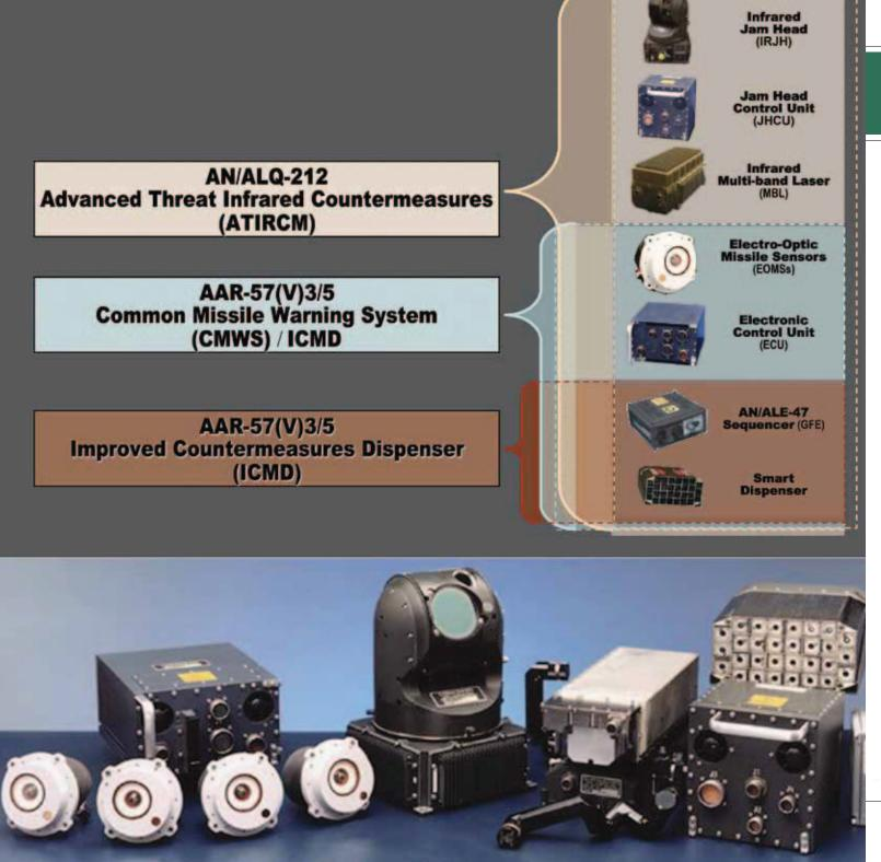
Advanced Threat Infrared Countermeasure/Common Missile Warning System (ATIRCM/CMWS)
