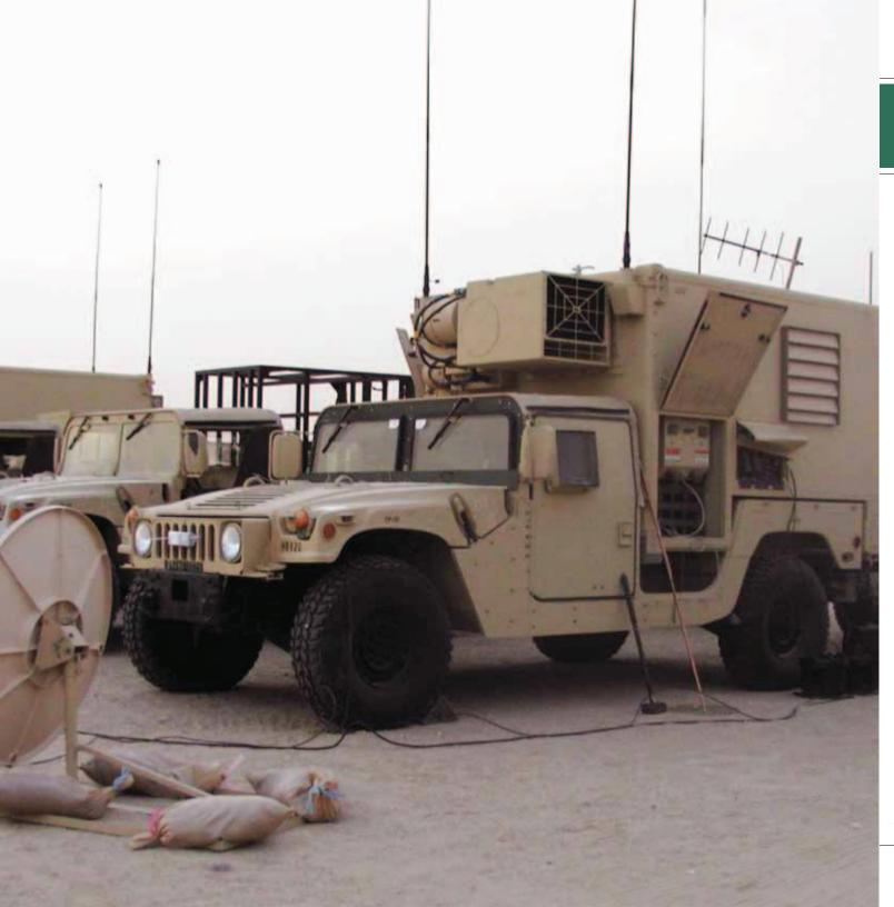
Meteorological Measuring Set-Profiler (MMS-P)/Computer Meteorological Data-Profiler (CMD-P)
