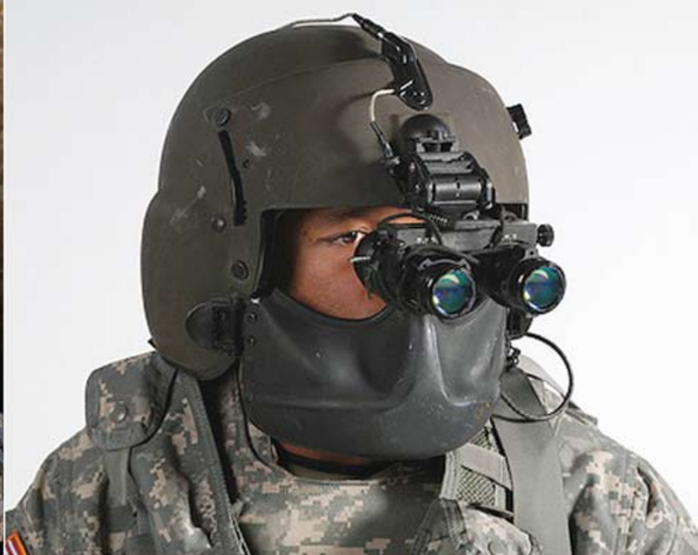
AN/PVS-14 Monocular Night Vision Device (MNVD)
