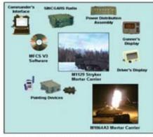
Mortar Fire Control System (MFCS-Mounted)
