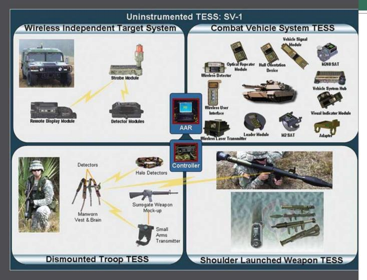
Instrumentable–Multiple Integrated Laser Engagement System (I-MILES)
