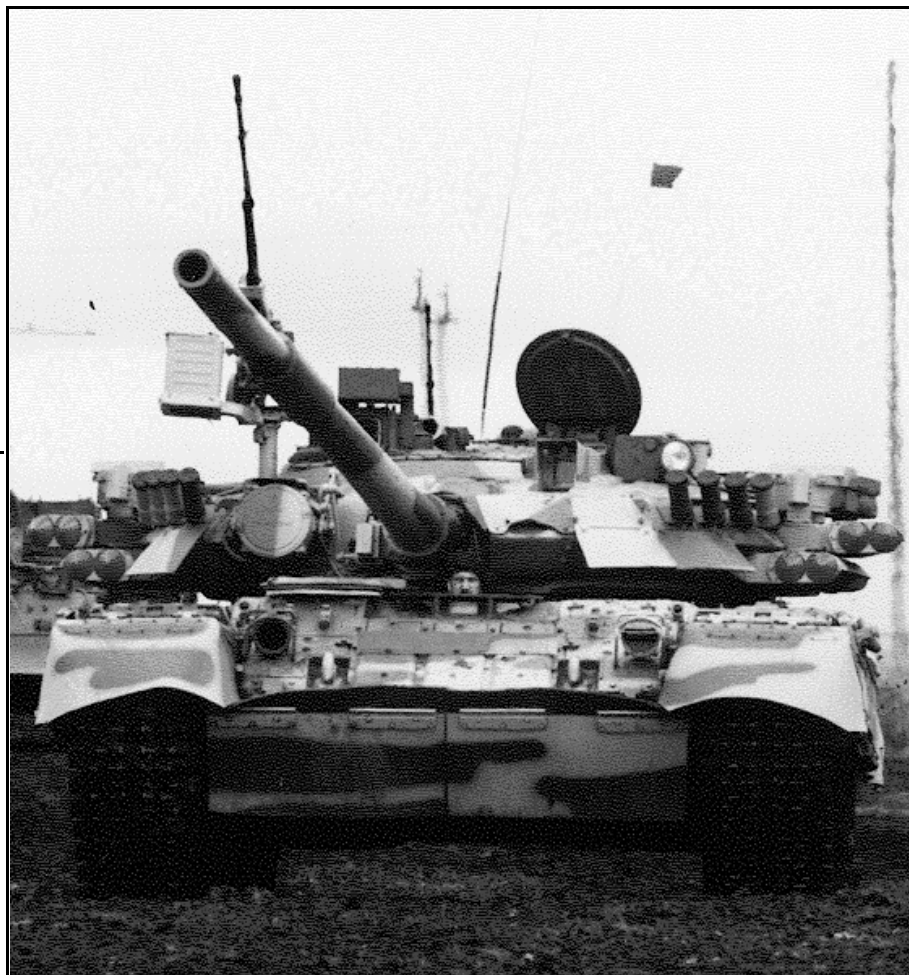
Drozd defensive launchers are visible at the outer edges of the turret, below and outside the smoke grenade launchers. Activated by a radar system that detects incoming rounds, the system's short-range self-defense rockets use fragmentation warheads. (All story photos taken at Omsk, Russia demonstration by Ron Dritelein of TACOM)
